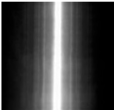
Fig.4. Isothermal kinematic electron diffraction pattern from amorphous TlIn_{0.92}Sn_{0.08}S_2 - II, undergoing a phase transformation at 438 K.
